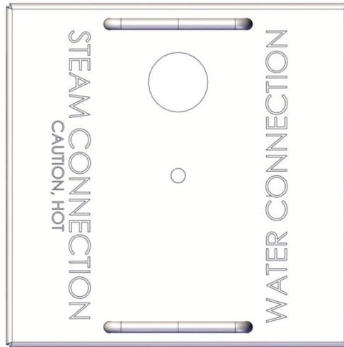
To make it easier for our customers the correct use of the Fortador Barrel Cleaner, we engraved the specific connections. **IT'S EXTREMELY IMPORTANT TO PAY ATTENTION** to where you plug in your machinery. Even though it is hard to confuse the two connections, **PLEASE PAY SPECIAL ATTENTION, DO NOT SWITCH THE STEAM CONNECTION WITH THE WATER CONNECTION.** By switching the connections, the Barrel Cleaner can be damaged, and what's worse, even the user can be hurt.
